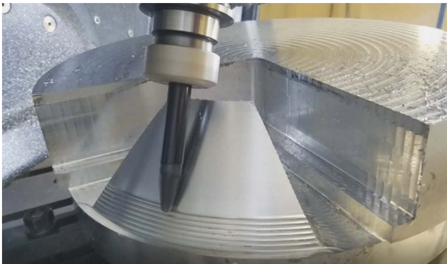
Barrel cutters, like this one from Iscar, can reduce finishing operations up to 60 percent in moldmaking operations, according to the company. Mastercam recently introduced the capability to recognize these special forms and create a toolpath using them along multiple surfaces. (Provided by CNC Software Inc.)
