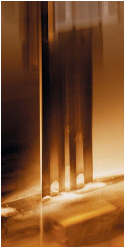
GF Machining's iGAP generator sensor technology helps moldmakers achieve a smaller, and therefore more precise, spark gap at higher speed with a die sinking EDM. (Provided by GF Machining Solutions)
