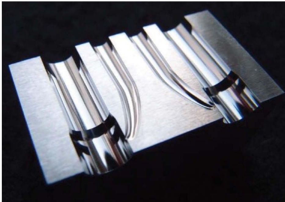
Direct milling of gates for injection molds like this banana gate overcomes some of the limitations of EDMing. (Provided by MC Machinery)
